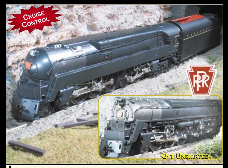
In its on-going quest to develop a truly efficient coal-fired express locomotive, the Pennsylvania Railroad introduced the opposed cylinder duplex Q1 in 1942. With 300 PSI and over 93,000 lbs. tractive effort, it was one of the most powerful non-articulated locomotives ever built and was the genesis for the even more powerful Q2 two years later.
